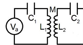
$$\frac{d^2 Q_1(t)}{dt^2} = \frac{1}{M^2 - L_1 L_2} \left[ \left( \frac{Q_1(t)}{C_1} - V_a(t) \right) L_2 + \frac{Q_2(t)}{C_2} M \right]$$
