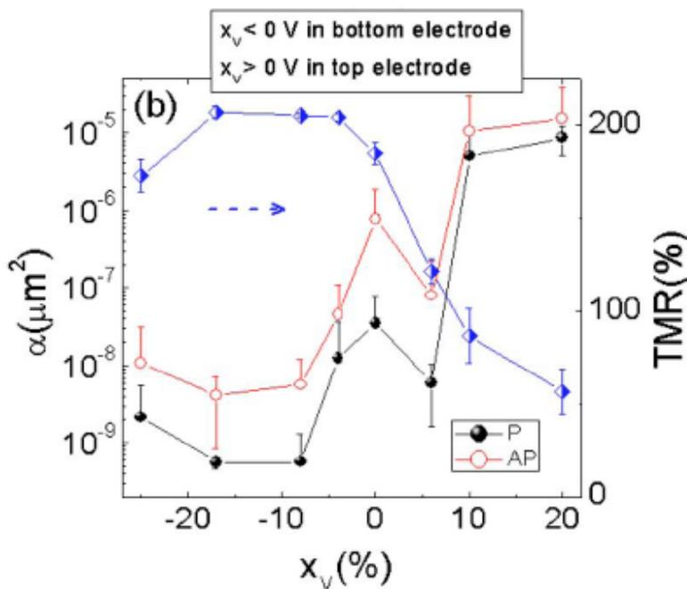
Alloying Fe electrodes with V, through reduced FeV/MgO interface mismatch in epitaxial magnetic tunnel junctions with MgO barriers, notably suppresses both nonmagnetic parallel and magnetic antiparallel state 1/f noise and enhances tunneling magnetoresistance. We attribute the enhanced TMR and suppressed 1/f noise to strongly reduced misfit and dislocation densit.
