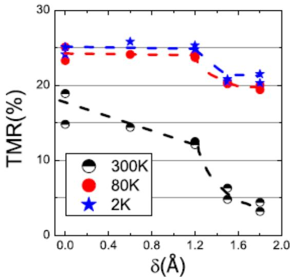
Dependence of the tunneling magnetoresistance on the silicon thickness at three different temperatures. While presence of silicon reduces significantly the polarization at room temperature, decreasing the value of the TMR ratio, for temperatures below 80K the presence of the silicon layer seems not to affect the spin polarization, for thickness below 1.2 Å.
