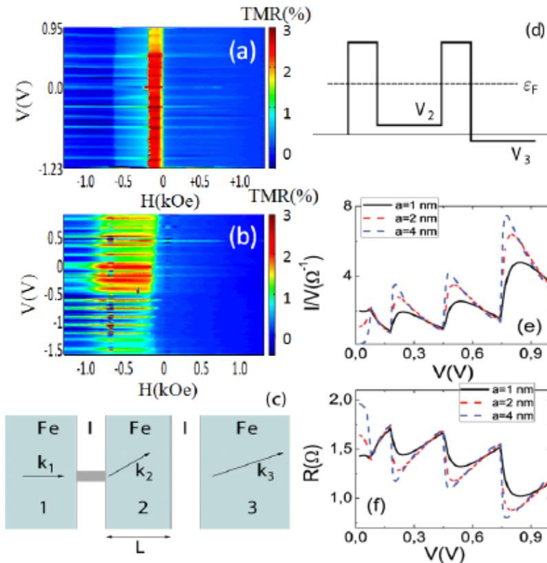
3D plot with magnetic field along  $x$ , bias voltage along  $y$ , and TMR along  $z$  directions. Panel (a) corresponds to magnetic field along the HA and (b) along IA. (c) Schematic presentation of the model with a single spot and (d) the corresponding energy profile. (e) Calculated conductance ( $I=V$ ) for DMTJ with a single spot in P state for different spot dimensions. (f)  $R$  versus  $V$  for DMTJ with multiple spots in the P state for different average spot dimensions
