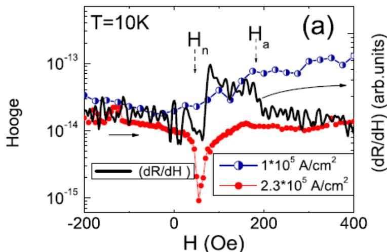
Dependence of the Hooge factor on the magnetic field for Fe/Cr MML obtained from noise measurements at  $T=10$  K with two different applied current densities. For comparison, the solid line shows the absolute values of the derivative  $dR/dH$ . The vertical arrows mark the regions of nucleation and annihilation of the domain walls determined from low field magnetoresistance measurements.
