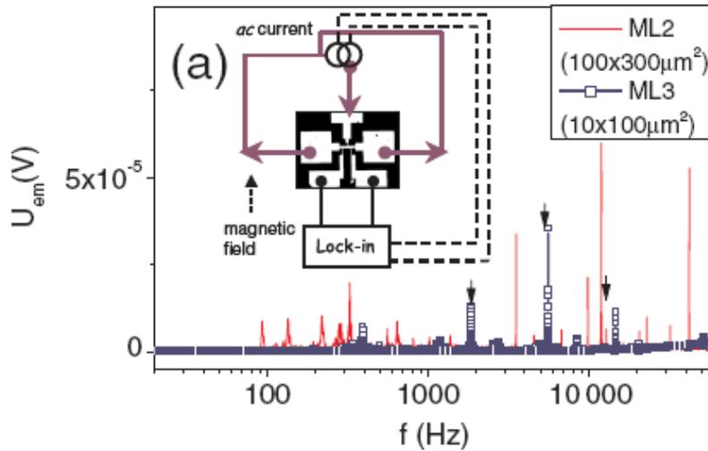
Frequency dependence of the voltage in 5 point geometry measured at 6 K for the in-plane field of 1T for two [Fe/Cr]10 on MgO multilayers with different dimensions. The inset sketches the five-probe measurement scheme.
