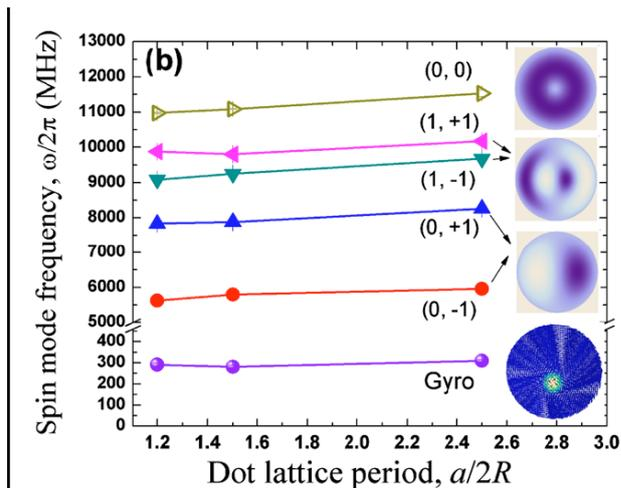
Zero in-plane bias field response of the three arrays of Py dots with different interdot separations,  $d=200, 500,$  and  $1500$  nm. The detected spin excitation frequencies labeled by the mode indices  $n,m$  vs the interdot separation.
