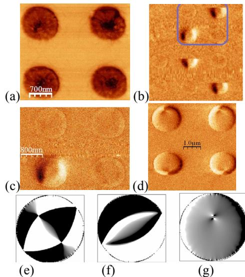
Figure 7: MFM images in zero field with commercial tip (a), with soft tip (b,c). Part (d) shows images of the shifted vortex in the field of 18 mT. Parts (e-g) present correspondingly simulated (within approach [15], in the absence of tip field) MFM images for DMV, S and shifted single vortex states.
