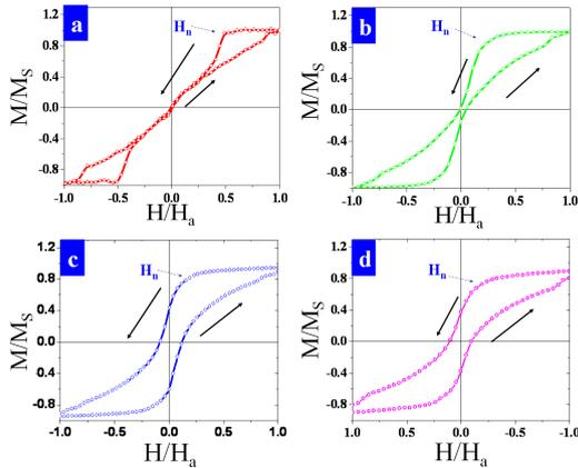
Figure 1 Hysteresis loops for the Py dot: a,b,c,d present the magnetization loops for dots with 1000nm diameter and 50, 25, 20 and 15nm thickness respectively.
