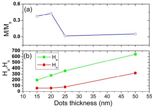
Figure 2 a) Normalized magnetization remanence  $M(0)/M_S$ . b) vortex nucleation and annihilation fields in Oe as a function of Py dots thickness.
