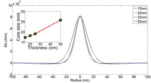
Figure 3: Numerically calculated variation of the vortex core size with dots thickness  $t$  (diameter 1036nm, cell size  $2 \times 2 \times t \text{ nm}^3$ ,  $T=0\text{K}$ ).
