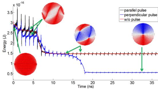
Figure 5 Relaxation of 1035x25nm dot with applied RF field that consists of a sum of sinusoids from 1GHz to 9GHz with amplitude of 100Oe. Saturated state, S-state, DMV state vortex state respectively as indicated by the snapshots of the magnetization at the indicated time, with a color coding for Mx. (dot: 1035x25nm at 60K).
