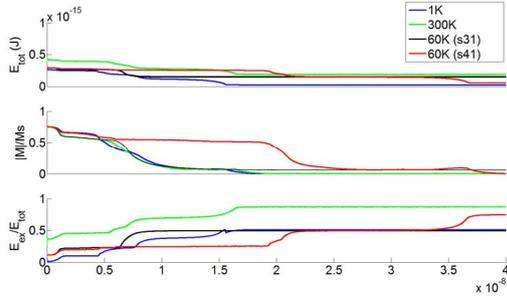
Figure 4: Relative energy contributions to the total energy vs. time for different simulated temperatures.
