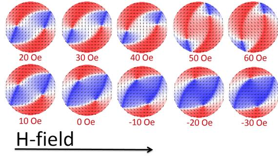
Figure 6: In-plane applied field parallel to the history field direction for dot 1035x20nm.
