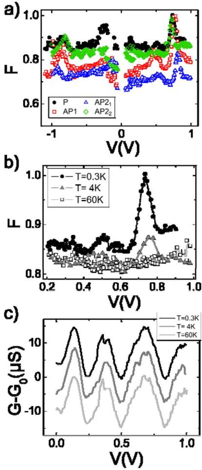
Fig. 3. (a) Dependence of shot noise with voltage for four different magnetic states. (b) Shot noise in the P state at 0.3 K, 4 K and 60 K. The effect of quantum well states is gradually suppressed with increasing temperature. (c) The oscillations in conductance due to QWSs are not affected by the temperature. The curves have been offset for better observation.
