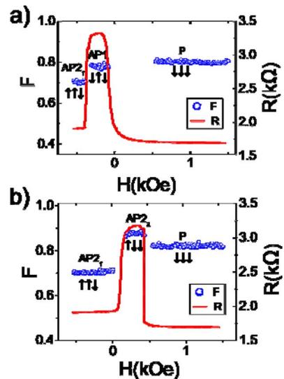
Fig. 2. Shot noise and resistance at a fixed current during a magnetic field sweep at  $T = 0.3$  K (a) from positive to negative values and (b) from the AP<sub>2</sub> at negative fields back to positive fields.
