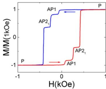
Fig. 1. Normalized magnetization hysteresis of the DMTJs, presenting three different magnetic states.
