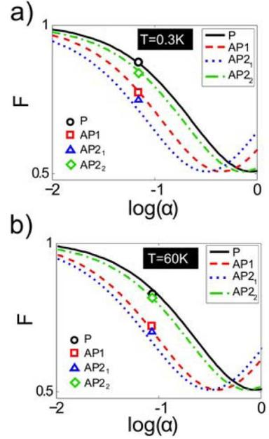
Fig. 4. Comparison of the experimental values (points) and the theoretical results (lines) for the Fano factors measured in the same sample at (a)  $T = 0.3$  K, with fitting parameters  $g = 100$ ,  $\alpha = 0.07$ ,  $\beta_1 = 5.7$ ,  $\beta_2 = 27.8$ , and (b)  $T = 60$  K, with  $g = 100$ ,  $\alpha = 0.08$ ,  $\beta_1 = 3.5$ ,  $\beta_2 = 28.3$ . The parameters  $\alpha$  and  $\beta_{1,2}$  describe the barrier asymmetry and the spin filtering of each MgO barrier (see [20] for details).
