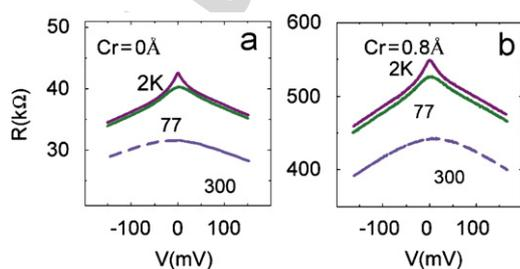
Fig. 1. Dynamic resistance vs. bias for undoped (a) and doped (b) MTJs measured between 2 and 300 K.
