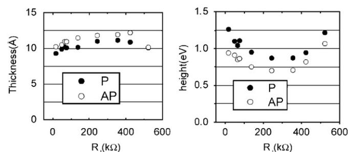
Fig. 2. Estimated thickness and barrier height for  $\text{Co}/\text{Al}_2\text{O}_3\langle\text{Cr}\rangle/\text{Py}$  MTJs. Resistance range separating doped and undoped junctions is shown in Fig. 4.
