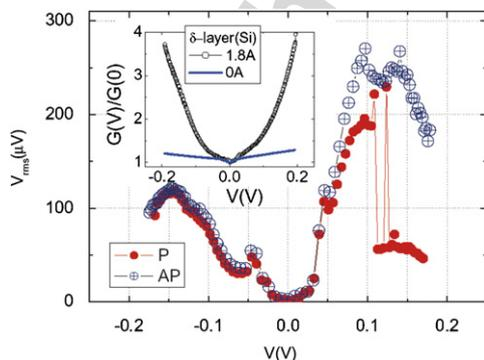
Fig. 5. Bias dependence of the  $V_{\text{rms}}$  and the normalized conductance in the P state (inset) measured at 2 K for MTJs with Si  $\delta$ -doped (1.8 Å) layer inserted asymmetrically. Inset shows the normalized conductance of the doped and undoped samples.
