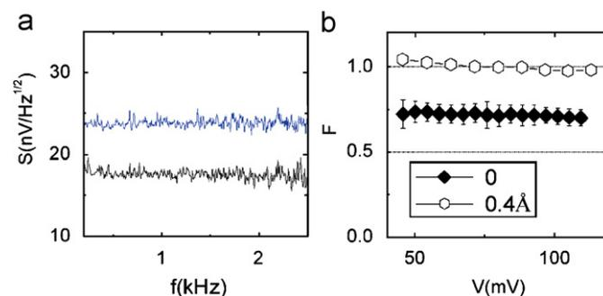
Fig. 3. Typical shot noise for currents of 3 and 6  $\mu\text{A}$  (a) and dependence of the Fano factor on applied bias (b) for two different MTJs measured at 2 K.
