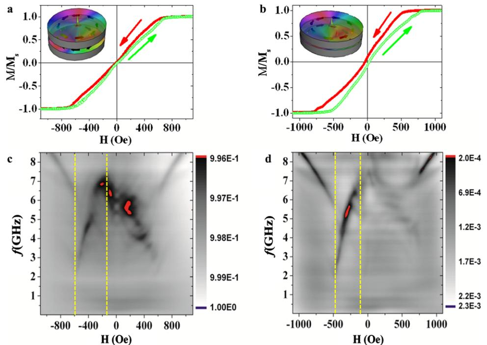
Here, we investigate, experimentally and by simulations and analytical estimations, the static and dynamic response of the vertically coupled Py dots with two spacer thicknesses, of 0.9 and 20 nm, in Py/Cu/Py nanopillars to external magnetic fields. We study the variation of both static and dynamic response between saturated and magnetic vortex states applying a bias in-plane field and compare the results with the spin wave spectra of uncoupled dots published previously [2].
